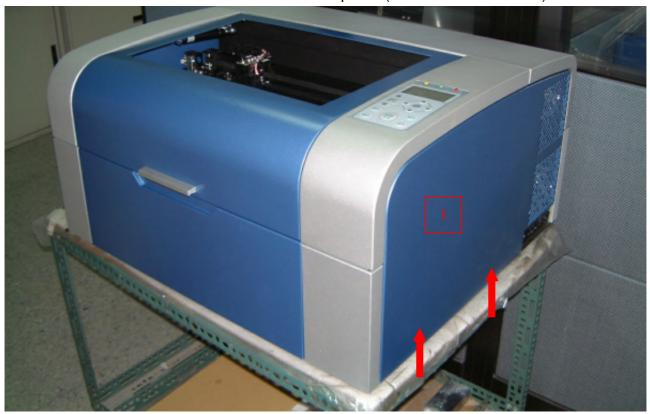
2. Dismount 7 screws (see red arrows below) and remove all cables connecting to main board and can change new main board.
