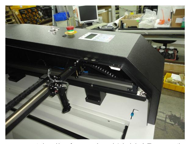
Then you can see control panel have four screws (see red circles below). Then remove the screws and unplug all cables and then change new one.
