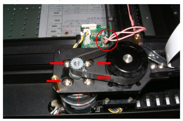
8-3 On lens carriage side, remove the auto focus cable also (it is tight, so use tweezers will be helpful).
