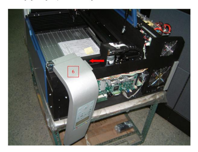
7. Dismount 5 screws for cover of control panel and ground cable screw
